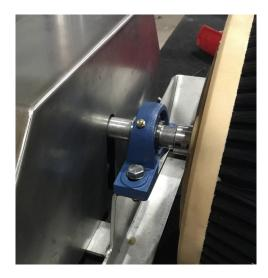
Each bearing house has a nipple for grease to be injected using a grease gun.
