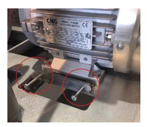
Loosen the 4 motor mounting base bolts for adjustments .
