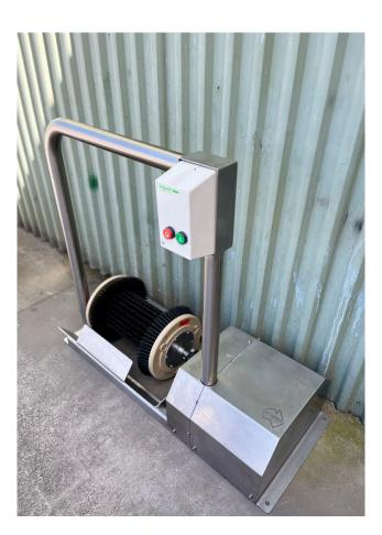
Inspect brushes for wear & ensure all bolts are secure. Check all bolts on machine are tight & secure. Ensure all bolts are tight on cover
