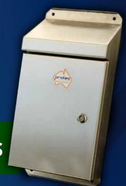
Our range of sloped roof enclosures are IP66 rated and come in a wide variety of siz Starting from (H) 300 x (W) 200 x (D) 150 mm up to (H) 1200 x (W) 800 x (D)300 Our Standard material is 2mm thick #304 Stainless Steel with other materials available on reque Enclosures come with optional left or right hinged doors.
