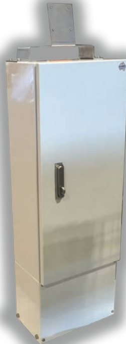
850x302x250mm Custom Enclosure w/ 300x302x250mm Plinth, Stainless Steel Swing Handle, Powder coated White, custom computer bracket mounted on top.
