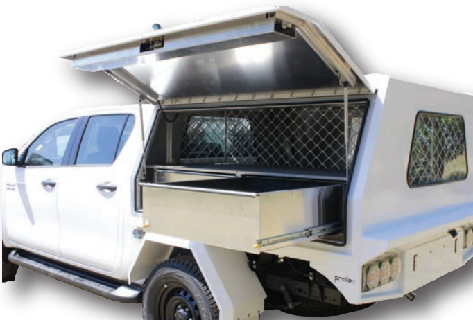
Powder Coated Stainless Steel with Aluminium Draws
